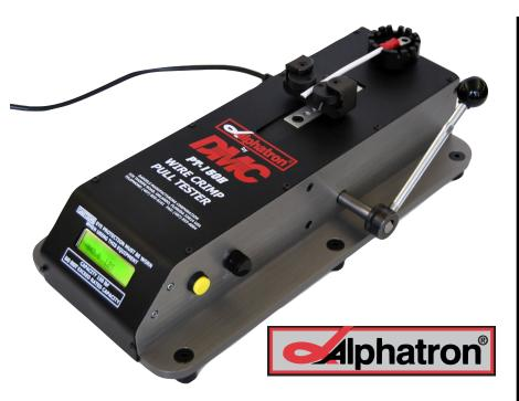
Now available from DMC is the PT-150H Electronic Manual Tensile Test System which may be used in conjunction with SPC Programs or other Quality Control disciplines in both OEM and maintenance applications. The electronic digital readout display is a fast and reliable source of test data.
